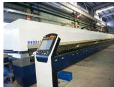
先进的超薄钢化炉 Advanced tempering machine for extra-thin deep processing
