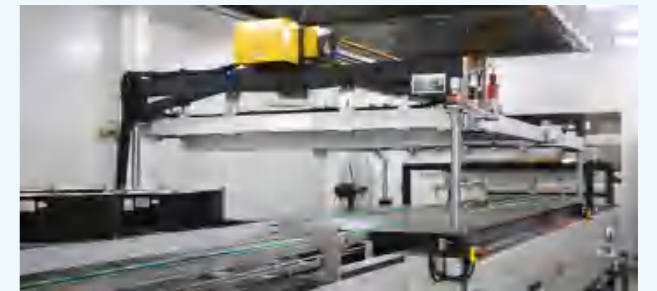
丝印机 Ceramic printing machine
